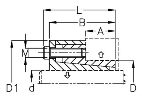
A mm = 14 B mm = 27.5 D1 mm = 40.5 d H8 mm = 14 D mm = 26 F kN torque = 14 L mm = 31.5 M mm = 4 P N/mm2 surface pressure on shaft/hub = 100 T N m torque = 90 Ts N m bolt tightening torque = 5
